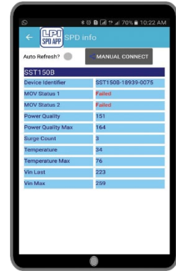
Replace as no protection is left
